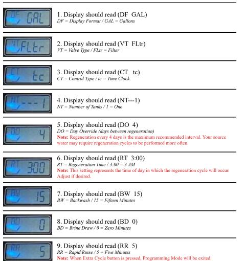
Display will revert to normal operation. Adjust the time of day to your current local time using the **Up** or **Down** arrows.
